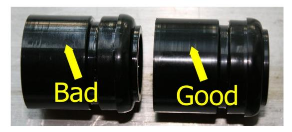
Additionally, in a side-by-side comparison the bad forward closures will feel more "slippery" to the touch than the good forward closures. However without a side-by-side comparison this will almost be unnoticeable. Again both of
